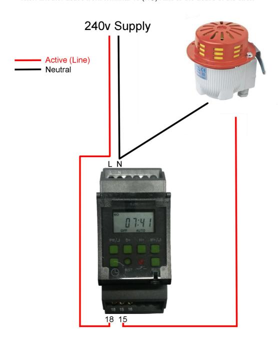
The green MAN button on the timer cycles between OFF, ON & AUTO. Choosing ON will activate the siren to test the connection.
